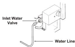
5. Remove control box cover and turn the timer into the harvest cycle.
